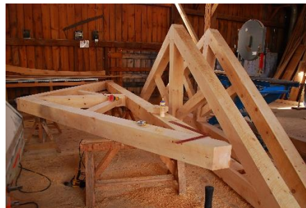
Structural Pine truss with concealed connectors
